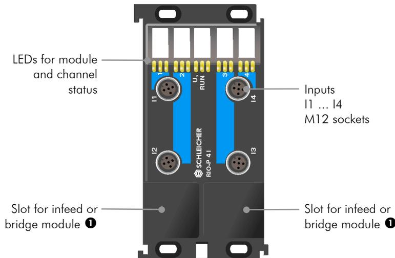
The RIO-P 4I digital module provides 4 input channels for binary DC signals with 24 V level. The inputs are suitable for sensors with NC or NO behaviour. The bus coupler outputs the data via the internal side bus and passes it, isolated, to the higher-level controller as a process map. The signal state of each channel can be read on an LED.
